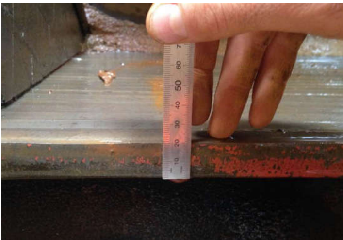
SPOT 60 OVERLAY LINERS AFTER 2 WEEKS – NO WEAR
