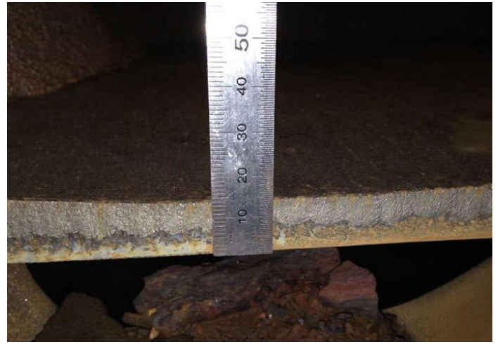
COMPETING PLATE AFTER 2 WEEKS – 4MM OF WEAR
